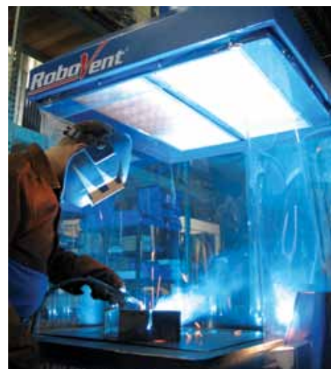
Model MOH-1200-1 RoboVent Canopy with optional clear curtain
